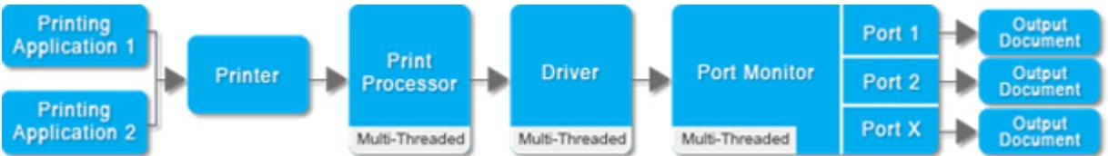
Designed for print server environments with simultaneous user printing, this configuration ensures performance similar to Parallel Multi-Printers but with a single printer. Perfect for scenarios like faxing or archiving, it provides a balance between performance and resource utilization.
