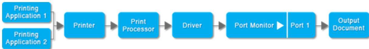
Ideal for single user low-volume printing, the Single Printer Driver offers sequential (single-threaded) printing, ensuring each queued document is printed one at a time. With low system requirements and CPU usage, this solution provides a simple yet effective approach to your printing needs.
