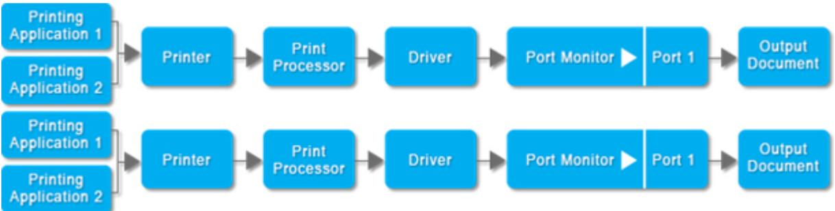
Tailor your printing setup with Complete Parallel Printers. Offering the same performance as Parallel Multi-Printers or Single Printer Parallel Drivers, this configuration provides separate printers, print processors, driver files, port monitors, and individual configuration INI files. Administrators can easily configure different printer settings, making it an excellent choice for integration with specific applications.
