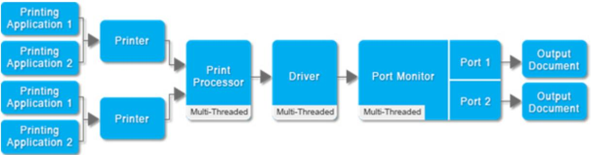
Our Parallel Multi-Printer configuration is the go-to solution for high-volume automated document conversion. Experience parallel printing and conversion, significantly reducing document conversion time. While demanding higher system requirements and CPU usage, the benefits of parallel printing make it ideal for efficient workflows.
